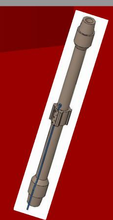
Operators need to have device that can be used to "quickly" clamp a wireline cable to a drill pipe and avoid the cable from slipping down and falling into the well.
